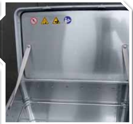
K470 after dust-tightness test.
